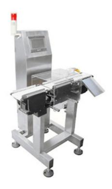
DMC High Precision Omnipotent Conveyor Weight Checker, can work with all kinds of packaging production line or equipment. In the process of dynamic drug delivery, DMC can realize the online weight test for all kinds of PE bottles, boxes, bags, tubes, PVC expansion sheet, penicillin bottle, cans and other packaging drugs in all forms and sizes, online sorting qualified products and unqualified products according to the pre-set weight range.
