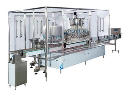
Glass bottle IV solution production line is mainly used for IV solution glass bottle of 50-500ml washing, depyrogenation, filling and stoppering, capping. It can be used for the production of glucose, antibiotic, amino acid, fat emulsion, nutrient solution and biological agents and other liquid etc.
