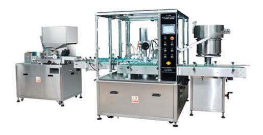
The liquid production processors design compliances with cGMP of the liquid product guideline. The processors are applicable for low viscosity and volume below 100ml.
