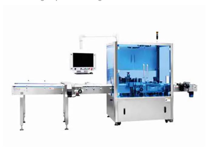
Wide conveying feeding  $\rightarrow$  spiral bottle dividing  $\rightarrow$  star plate feeding  $\rightarrow$  batch printing and pasting  $\rightarrow$  label online detection and rejection  $\rightarrow$  finished product  $\rightarrow$  unloading bottle clamping. This equipment is suitable for labeling small round bottles made of glass, plastic and metal (such as oral liquid bottles, ampoules, penicillin bottles, solid rubber bottles, plastic round bottles, etc.).
