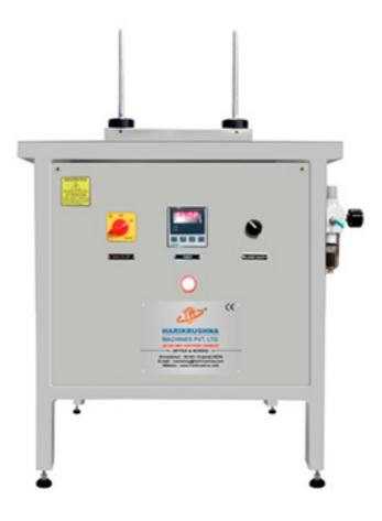
The Semi-Automatic Air Jet Vacuum Cleaning System consists of main structure, Ionizer, Air Nozzle, foot operated switch and Vacuum Suction Blower by HMPL.
