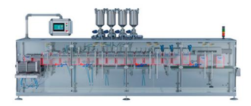
This series of horizontal pouch double-outlet packaging machines is a fully automatic prefabricated pouch packaging machine with a speed of 70 pouch/min, which is suitable for the packaging of flat pouchs and independent pouchs to achieve high-speed and economical packaging solutions. suitable for powder, particle, liquid, paste, solid, and other material packaging needs.
