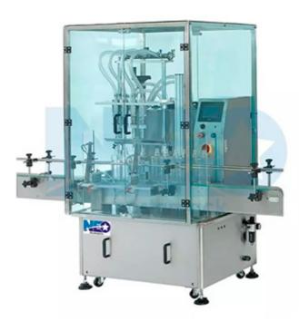
Automatic overflow liquid filler with safety gate FL5250 is designed for mineral water filling requirement with massive volume. The liquid level of every bottle will be the same and the surplus bubbles will overflow to reservoir. It especially suits for foamy liquid.
