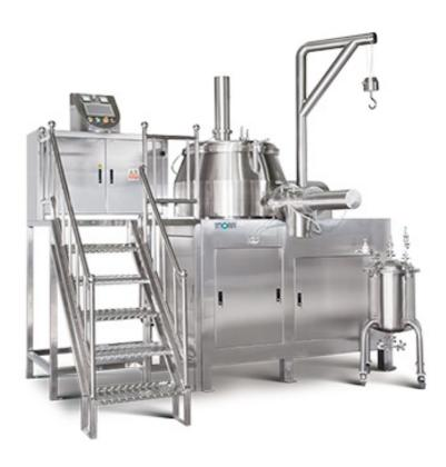
Super mixer granulator, also called Rapid mixer granulator RMG, is suitable for the high speed dispersion of dry powders, aqueous or solvent granulations. Rapid mixer granulator provides perfect mixing in short time for wet granulation process. In high shear granulation, dry powder is mixed in a bowl using impeller that spins powder into a vortex.
