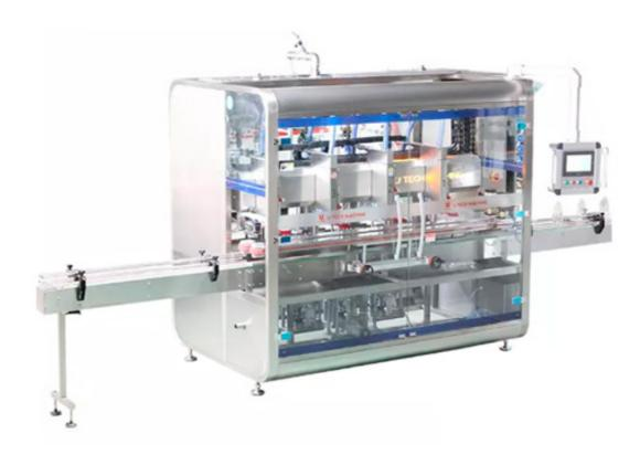
This UT series automatic edible food oil filling machine for bottle adopts serve ball-screw system to drive the piston cylinder. It's widely used in Food, Chemical, Medical, Cosmetics, Agrochemical industry, applicable for filling liquid, especially for high viscosity material and foamy liquid, such as: Oil, Sauce, Ketchup, Honey, Shampoo, Lotion Lubricant oil, etc. And it is suitable for barrels, jars and bottles of different sizes, shapes and volumes.
