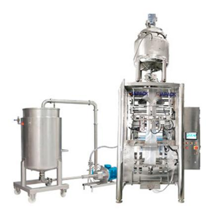
This machine unit are special design for packing small sauce product like ketch up, chili sauce, Fish meal and so on. The machine can automatic make the bag, weighing the product, filling product in to bag and then output the conveyor. The whole machine are control by PLC and can operate on Touch screen. Easy for adjusting and maintain.
