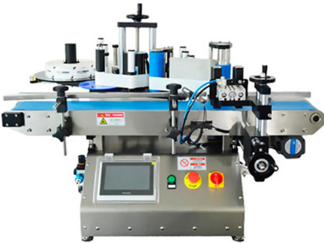
This Desktop Automatic Round Bottle Labeling Machine is designed for high-precision labeling of cylindrical containers, such as bottles and jars, in a compact and efficient tabletop format. It is ideal for industries such as food, beverage, cosmetics, and pharmaceuticals, where precise label placement is essential.
