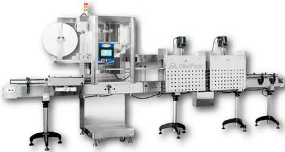
The automatic shrink sleeving machine from Allen Pack can easily be integrated with your company's existing packaging lines or we can also provide a complete system which would include the applicator, conveyor, and heat tunnel. It's suitable for all bottles with various width range and label position application.
