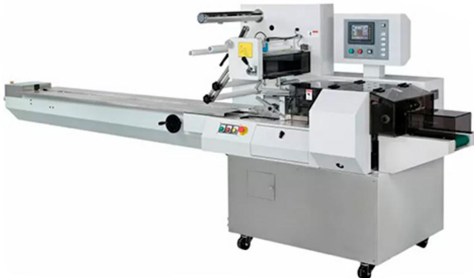
The digital horizontal packaging machine features a 5.7-inch microcomputer HMI touchscreen, allowing easy control and operation. It can store packaging parameters such as temperature, bag length, and packaging speed, with memory capacity for 50 or 100 sets of settings. The machine is designed for easy maintenance and can be integrated with basic automation systems to enhance performance.
