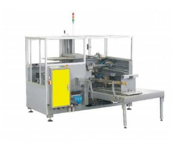
Case erectors and case cartoners are case equipment which automatically forms corrugated cases. A stack of corrugated blanks are knocked down and placed into the machine. The blanks are pulled out of the machine one-by-one and formed into cases. The newly formed cases are sealed at the bottom with tape or glue.
