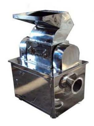
The machine is applied as supporting equipment, before rune crushing process in trades as pharmaceutical, chemical and foods ruffect it specially grinds the hard and solid granule materials like plastic materials and cooper wires. Also it can be the pretreatment coordinated machine for fine grinding process
