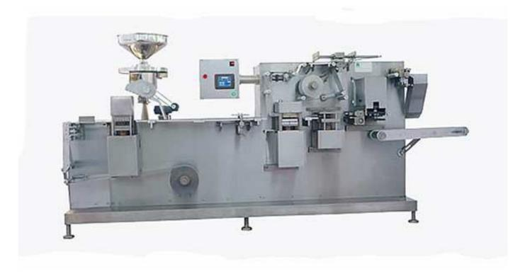
Blister packing machine is suitable for both the Cold Forming and thermo forming blisters. The machine is suitable for large batches.
