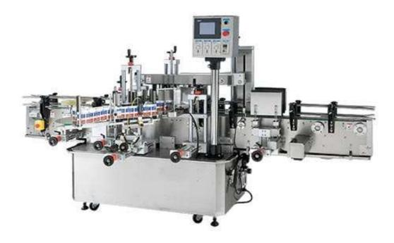
KWT-600 serials are manufactured for front and back sides of square, rectangular or oval containers as well as circular ones (wrap around).
