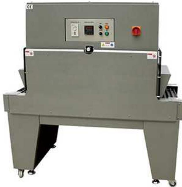
1. Double furnace design, the furnace is divided into two temperatures, and the temperature can be controlled separately.
