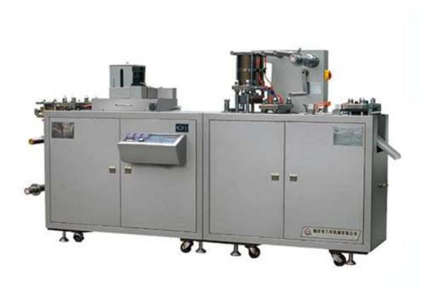
Blister Packing Machine is on the basis of DPP-250F and widely absorbing the feedback information from customers and the advantages of same-type products at home and abroad. It is strictly made conforming to "GMP" standards. A waste material collecting device has been designed to add up to this machine which can make the function of the whole machine more perfect.
