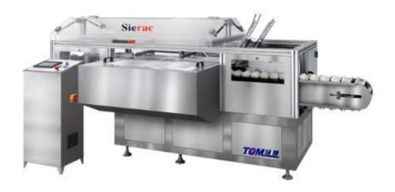
The new series cartoning machine built with "BALCONY" design, allowing the mechanical working parts separated from the packaging area. It respects the present accident prevention maintenance and hygienic laws. The machine works with intermittent motion and with electric synchronisms controls, PLC and touch display control system functions recall-able; it is possible memorizing 100 menus with relative data for 100 different productions.
