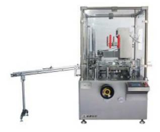
This machine is suitable for cardboard case packaging of blister packing for impulse, injection. It consists of direction folding (1-4 folds) and feeding equipment, cardboard case forming and feeding, batch number printing, sealing of case tongues at both ends ect. The whole encasing process is finished automatically. It can be added hot-glue machine.
