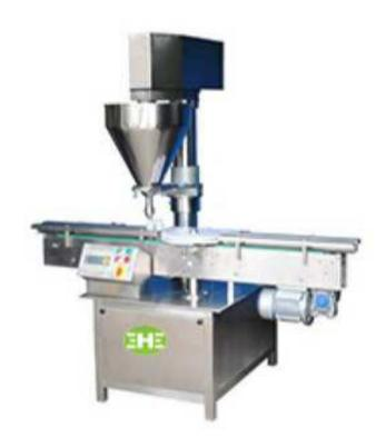
Single Head Auger Powder Filling Machine is used to fill variety of product like granules, powder etc in bottle. It basically works on Auger base to fill powder in bottle.
