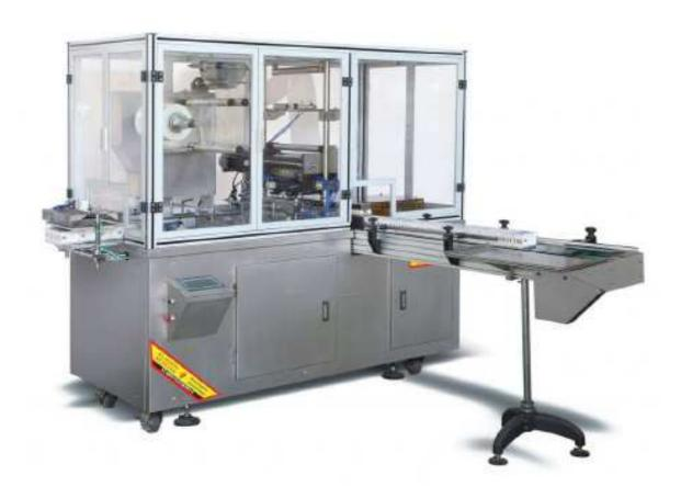
This Cellophane Wrapping Machine is suitable for cellophane and BOPP film coating, for different specifications of cardboard packaging boxes, packaging products for three-dimensional packaging equipment.
