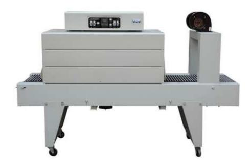
The shrink wrap machine is suitable for all kinds of shrink films. The shrink wrap machine adopts digital temperature controller, which makes operation easier. There are shrinking tubes on the top, bottom and sides of the shrinking room. The powerful fan inside the tunnel makes the air heating equally. The speed of the conveyer is adjustable. And you can choose roller or net conveyor as your request.
