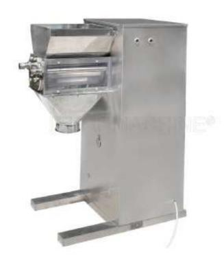
This machine is used mainly in such trades as pharmacy, chemical industry, food, pottery and plastics extensively, making moist powder material particle. Make cylinder swing reciprocatly, extruding material from screen mesh for granulation. It also can be used for crushing the agglomerate materials into small granules directly.
