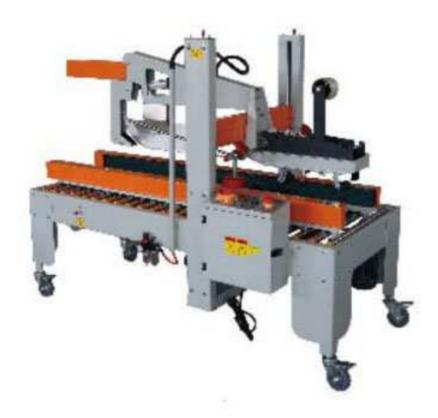
A case sealer or box sealer or carton sealer is a piece of equipment used for closing or sealing corrugated boxes. Fully automatic equipment is available which does not require an operator. All functions, including closing the flaps, can be automated.
