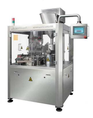
NJP-2800 empty medicine capsule filling machine is designed for large-volume production based on the NJP 2200. As ideal processing equipment for hard capsule pharmaceutical factory, new powder vacuum recovery unit, safety protection device for human and machine and automatic shutdown device are used to ensure smooth running, safety and reliability.
