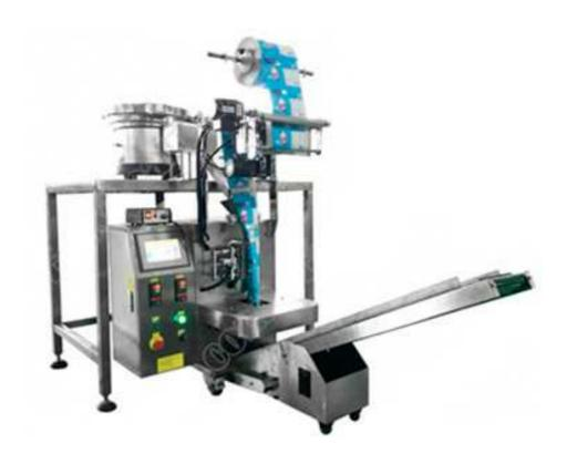
This automatic counting packing machine, is suitable for milk tablet packaging, pill and tablet packaging. It completes tablet piece counting, filling, bagging with high precision.
