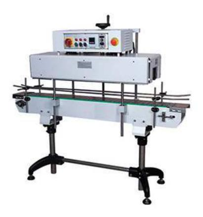
The SM-1540 cap label shrinking machine only heats and shrinks the part of bottle mouth, saving heat energy and not affecting the quality of the objects in the bottle due to temperature. The use of double small power transmission wind turbines, does not cause the label to shift and deform. The height of the furnace is adjustable and can be applied to a variety of bottle types. The SM-1540 cap label shrinking machine can be used in stand-alone operation or in conjunction with production lines.
