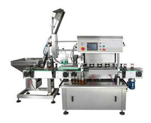
Automatic twist off glass jar vacuum capping machine is used for tinplate caps' vacuumizing and capping in glass jars. It integrates automatic caps arrangement, automatic caps loading, automatic vacuumizing and automatic capping into one machine. When there is no bottle, there will be no caps sending, and when there is lack of caps, the machine will have an automatic alarm and it also has other functions.
