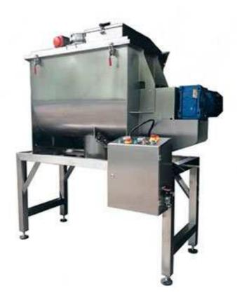
The ribbon mixer machine consists of a U-shape tank, spiral and drives parts. The spirals dual structure. Outer spiral makes the material move from the sides to the center of the tank and the inner screw conveyor the material from the center to the sides to get the convective mixing.
