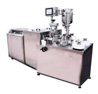
It can complete making shell forming, filling, condensation and sealing. The machine is made of PLC, HMI, because of its full-featured, small volume, low production, so it is used for research institutes and hospital preparations
