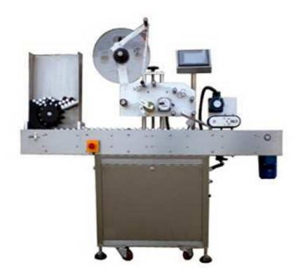
This machine adopts fully-mechanic drive that is made up completely sealing oiling boxes of high smoothness, few troubles and small noise. The motor load is low, the panel, and running disc transmission strap are made of stainless steels that are endurable, clean and easy to maintain. It occupies small space and can be moved freely in the work place. The use of paste labeling machine can greatly lower the cost for labeling.
