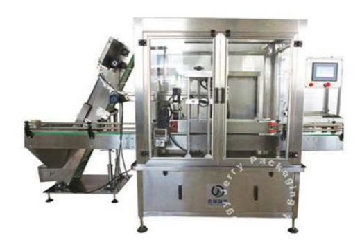
The JCP-35 innovative and highly efficient design enables easy operation and quick change-over for different capping specifications and requirements. Especially its new continuous style pick & placing function which drives by triple servo motors can exactly make sure all the caps can be capped precisely and tightly on the products.
