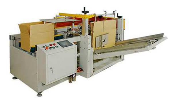
Automatically complete the top and bottom folding, while simultaneously completing the upper and lower two parts of tape at the same time, saving labor and time.
