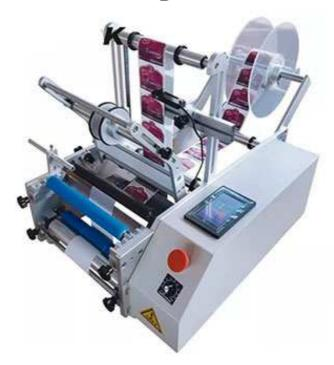
The LT-190-I Round bottle labeling machine, is suitable for cylindrical object labeling of various specifications, which can realize full week/half week. labeling/circumference front and back labeling; The space between front and back can be adjusted arbitrarily;
