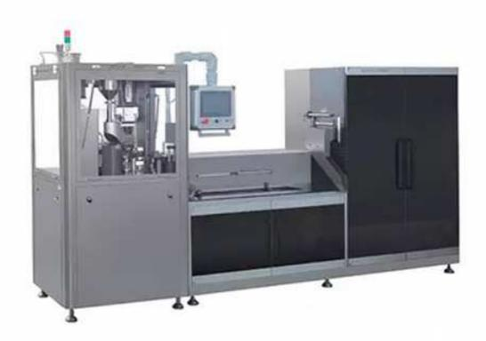
NJYF-300C automatic hard-capsule liquid filling machine and sealing linkage line equipment are the first in-line equipment of our company based on our own multi-year capsule filling technology, self-developed design and production of hard capsule filling liquid and sealing.
