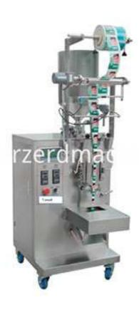
This liquid sachet packaging machine is suitable for the three-side and four-side sealing packing of liquid materials.
