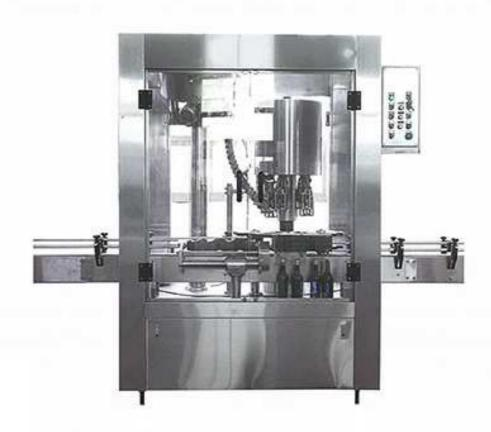
The rotary capping machine adapts 2 capping or snapping nozzles for packaging lines. It is flexible and durable and works with most containers and caps including flat caps, sport caps, metal lids and so on.
