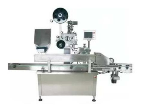
WTB-C is economical, self contained, easy to operate, equipped with auto PLC and touch screen. Built in microchip storing different job setting makes fast and easy changeover. This automatic labeling system is combined with bottle to tray inserter, it is ideal for slim cylindrical container with different from 10mm-25mm such as ampoule, small vials.
