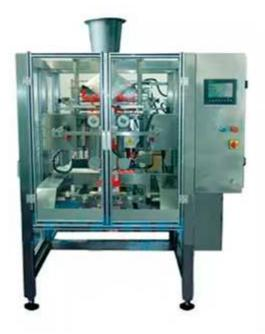
VFFS-5000 GD automatic VFFS packaging machine can make three-side sealing bag such as pillow bag, ruffled bag, hole-punching bag, etc. This machine can pack granule, powder, flaky material, pelletized material and irregular material when equipped with different kind of weighing machine.
