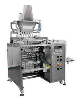
Automatically measuring volume, making bags, filling, sealing, cutting, printing the lot number and cutting easy tearing notches, finished product conveying.
