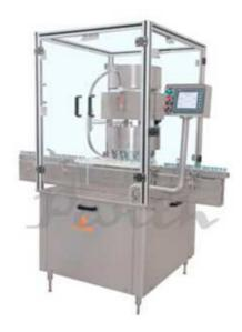
Automatic VIAL Cap Sealing Machine is versatile, self-supported on stainless steel leg with height adjustable adjustment system. The machine is precision built on sturdy welded MS frame completely enclose in stainless steel sheet and doors are providing to facilitate the servicing of machine.
