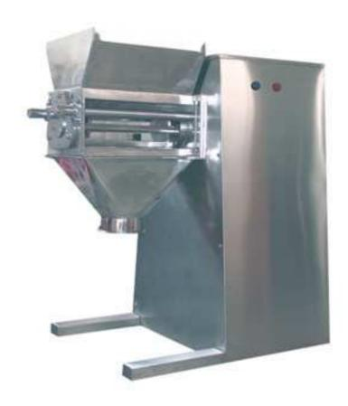
Under the positive and reverse rotation of the rotating drum, this granulator machine force the wet powder mixture through the screen to make granules.
