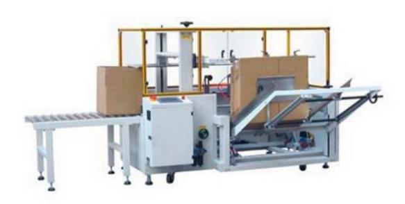
The working process of the carton erector is open the carton, carton in shaped, bend the carton bottom and seal the bottom with adhesive tapes. After the carton bottom is bend and sealed, it will convey to the carton packing machine. The carton erector is widely used in the automatic carton packing industry. The whole process is controlled by the PLC and touch screen. It is a necessary part in the automatic packing process
