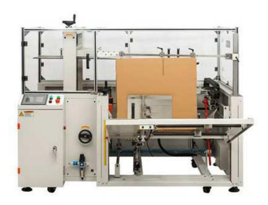
Suitable for carton sealing of the same specification at the same time; simple operation, convenient use, easy adjustment, fast unpacking speed, high efficiency, ruggedness, can be used stand-alone, and can also be used in conjunction with the packaging line after automation.
