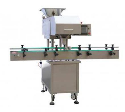
GS-8 Tablet capsule counter is an auto counting machine equipment which adopts advanced vibration and 8 channel, computer control, dynamic scan counting automatically. Candy Counting Machine with compact design is comply with the standard of GMP. Candy Counting Machine is easy to be operated without training. Compose the light, electric machinery to one set, which is suitable for tablet or capsule counting and filling in lab, semi-works.
