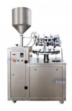
This semi-automatic tube filling sealing machine is quantities filling for the material of food, daily chemical, chemical, medical packing etc. Such as, food gel, cosmetic cream, face cream, hair dye, facial cleanser, ointment, resin, shoe polish and AB glue etc.
