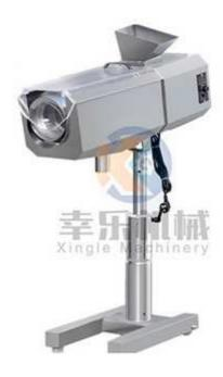
The tablet sieving and conveying process is completed inside a sieving box with a closed structure. When it works, the sieving box and material inlet and outlet are under negative pressure status without dust emission. The sieving box and power box are totally isolated from each other. The quick disassembled structure makes it convenient to disassemble, install and clean the machine.
