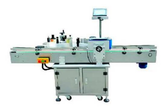
Applicable labels: self-adhesive label, self-adhesive film, electronic supervision code, bar code, etc.
